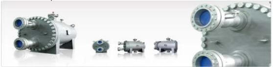
SEC Plate & Shell Heat Exchangers are an extremely efficient design primarily due to the high turbulence created by the strategically designed geometry of the plates. These turbulence allow very high heat transfer co-efficients. These values equate to less required heat transfer surface for any given heat transfer duty. Therefore, the end result is a compact, cost effective heat exchanger.
